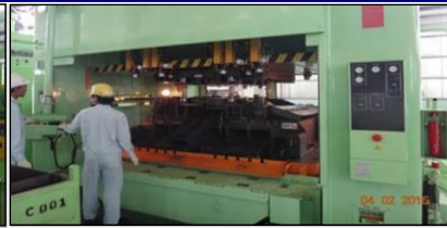
PRESS MACHINE-No.1 HP800ton
