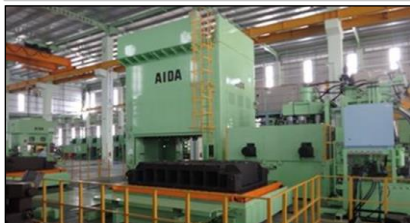
PRESS MACHINE-No.3 BIG TDM LINE (600tonX1-400tonx3)
