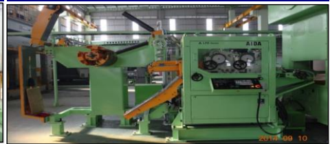
PRESS MACHINE-No.2 HP200ton
