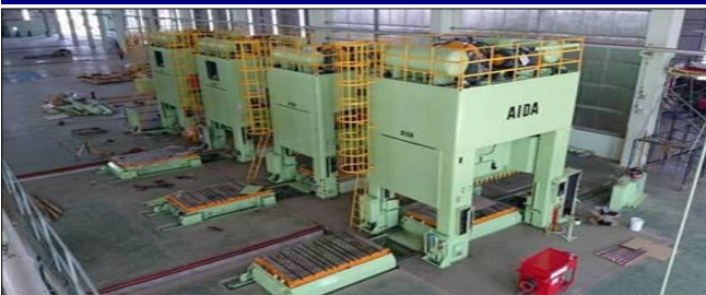
PRESS MACHINE-No.3 BIG TDM LINE (600tonX1-400tonx3)
