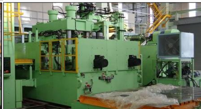
PRESS MACHINE-No.3 BIG TDM LINE (600tonX1-400tonx3)
