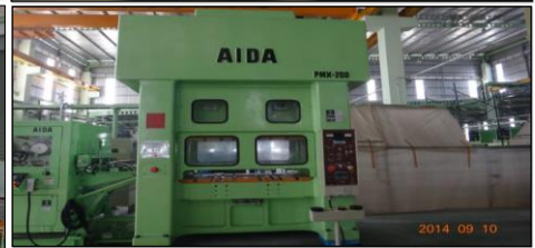
PRESS MACHINE-No.4 SMALL TDM LINE (200tonX1-150tonx2-110tonx3)
