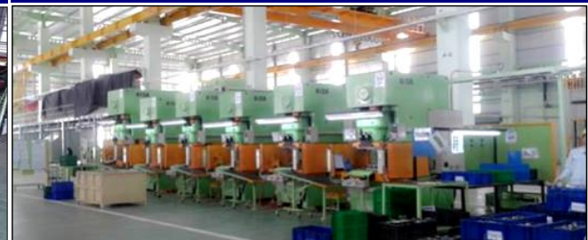
PRESS MACHINE-No.4 SMALL TDM LINE (200tonX1-150tonx2-110tonx3)
